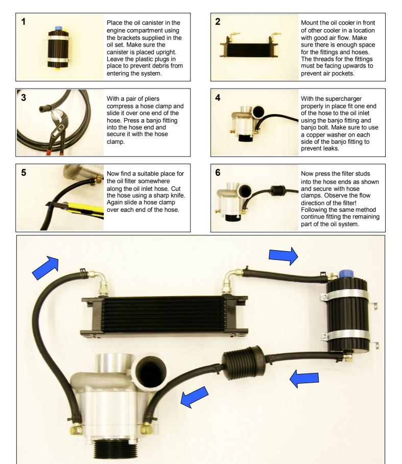
The finished oil system shown above with oil flow direction as indicated by the arrows: Oil flow from the oil canister through the filter into the compressor oil inlet. The compressor oil outlet routes through the cooler before entering the oil canister at the top.
